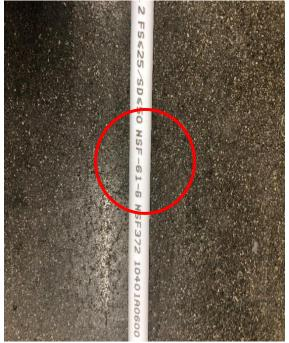
PEX Potable Water line with NSF- 61 label
